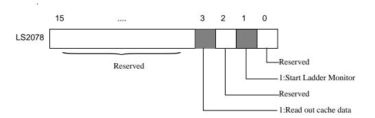
Bit 1:Turning this bit ON starts the Ladder Monitor. The Ladder Monitor menu will not appear.
