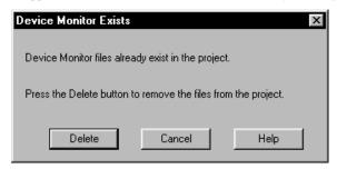
Click [Delete] to delete the currently registered Device Monitor data. Then, select [Screen / Setup] menu's [Device Monitor], and click [Add] to register the feature again.
